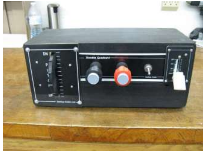
Trim, throttle/mixture & flap controls, in housing built by Larry Bothe, awaiting installation on the museum flight simulator.
