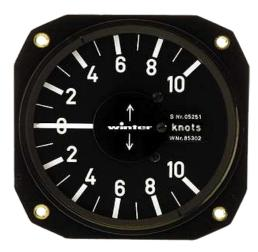
A positive rate shown on the TE vario indicates the glider is gaining energy. Conversely, a negative rate indicates the glider is losing energy. As we'll see later in this article, the TE vario might show 4 knots up when the glider is flying straight and level. (Note: 1 knot is roughly 100 feet per minute.) Therefore, the face of a TE vario might have the appearance of a VSI, but the needle behaves very differently.
