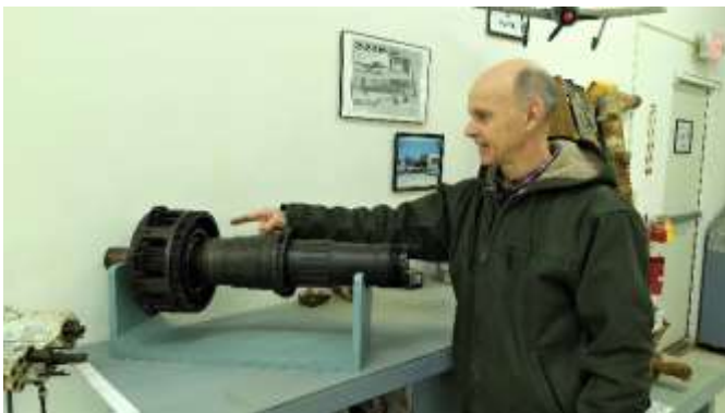
Museum president Joe Clegg with new BMW 801 prop shaft and planetary gear display.
