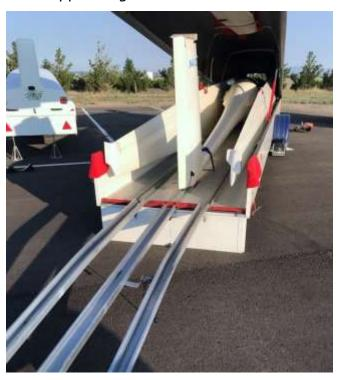
The first step in disassembly is maneuvering the fuselage into a cradle (at the rear of the trailer) that'll provide support as the tail surface and wings are removed. Once the glider is secure and there's no chance of shifting, it's time to carefully remove the horizontal stabilizer and wings. Support stands are used to gently lift the wings to support their weight. With the correct upward pressure, the main wing pins are easily removed. Removing or installing wing
