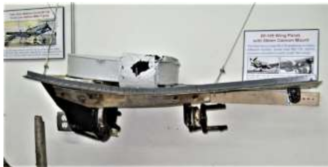
Wing panel from German Bf-109, with 20mm cannon mount below & ammo drum above.
