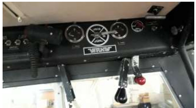
Mixtures (red), Throttles (black) and Carb Heat (white) in the front cockpit, left side. There is a duplicate set in the rear cockpit.
