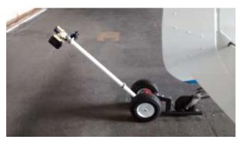
It is powered by a DeWalt 20v electric drill. The drill has plenty of power to move the plane, but what we have learned so far is that it takes an uncomfortable amount of force to push down on the drill and handle to lift the tailwheel up to move the plane. We have an optional 18" longer (48" instead of the 30" one in the picture) tube/drive shaft on order. I'll let you know next month how that works out.
