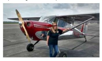
The airplane started as a Cessna 120 fuselage, the wings were changed to Cessna 150 wings, but with the flaps removed to save weight, and with the long-range Pipeline Patroller fuel tanks. It has a single wing strut on each side; not sure what they are from, maybe custom fabricated. The landing gear is Cessna 140. The engine is a Continental C-90 (stock Cessna 120/140 engine near the end of the production run) with a Sensenich wood prop (half the weight
